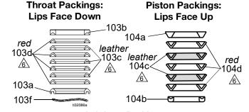
Lubricate Packings (soak leather packings in oil for 1 hour)
