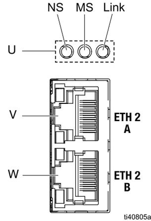
Fieldbus LEDs (U) are listed below from left to right, for both **EtherNet/IP**, page 19, and **PROFINET**, page 20.
