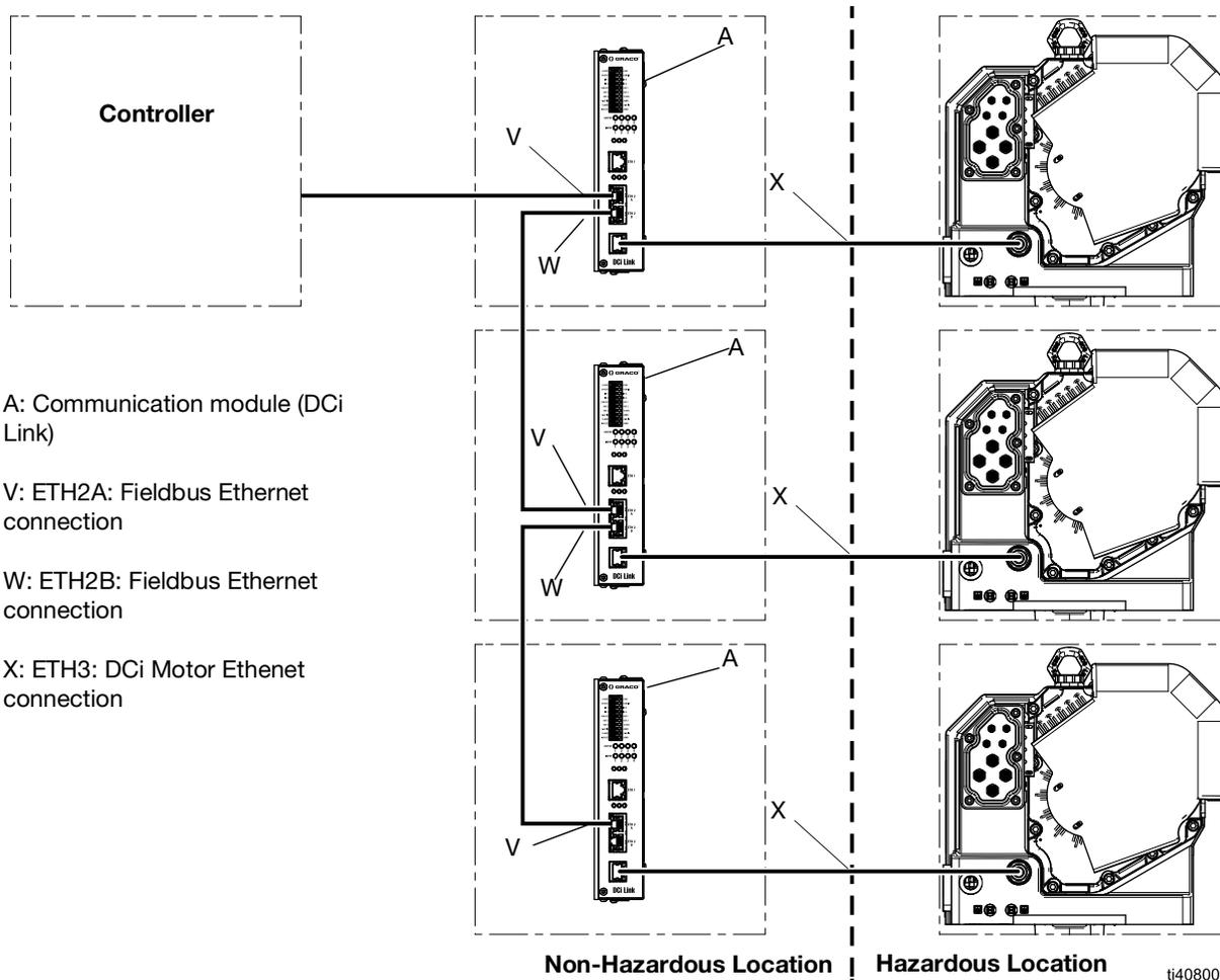
**FIG. 9: Daisy chain installation**
