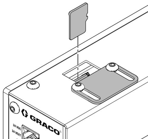
**Fig. 50: Replace the SD Card**
