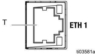
2. Insert the other end of the Ethernet cable into a computer with an updated operating system.
