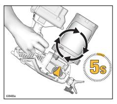
e. Turn sprayer upright and open the VacuValve Cap.
