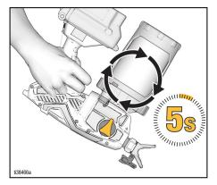
Rotate Spray Tip 180 degrees to UNCLOG position. Turn Prime Knob forward to SPRAY position.
