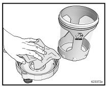
20. Wipe disinfectant off the outside of the sprayer using a soft cloth moistened with water.
