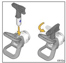
Screw Spray Tip Guard assembly onto sprayer and hand tighten.
