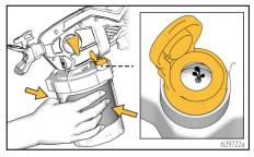
h. While continuing to squeeze the FlexLiner, close the VacuValve cap.
