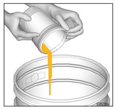
6. You can either dispose of the used FlexLiner and install a new FlexLiner, or clean a used FlexLiner. 7. Fill FlexLiner with warm water.
