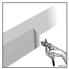
Trigger gun after moving. Release trigger before stopping. For additional spraying information, see separate gun manual.
