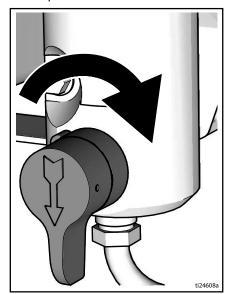
Place fluid intake with drain tube in grounded metal pail partially filled with flushing fluid. See Grounding, page 11.
