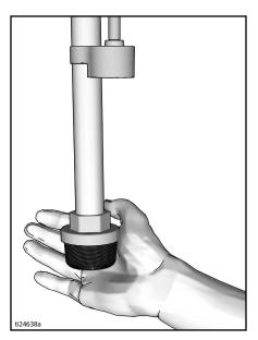
Fill throat packing nut with TSL to prevent premature packing wear. Do this daily or each time you spray.
