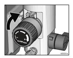
6. Turn prime valve horizontal. Disengage trigger lock.
