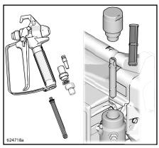
If flushing with water, flush again with mineral spirits or Pump Armor to leave a protective coating to prevent freezing or corrosion.
