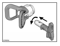
3. Screw assembly onto gun. Tighten.
