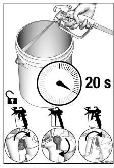
Inspect Airless Hose and hose connections for leaks. If leaks occur, perform Pressure Relief Procedure, page 12, then tighten all fittings and repeat Startup procedure. If there are no leaks, continue with Operation, page 19.
