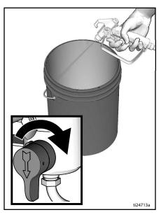
9. Raise fluid intake above flushing fluid.
