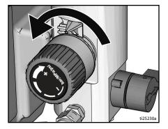
3. Turn ON/OFF switch to ON position.
