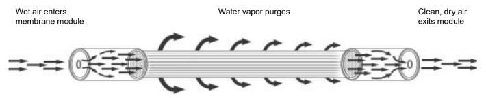
Water vapor permeates through hollow membrane fibers
