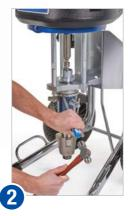
Loosen the jam nut
