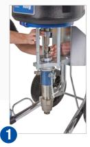
Remove rod coupling, inlet hose and paint
