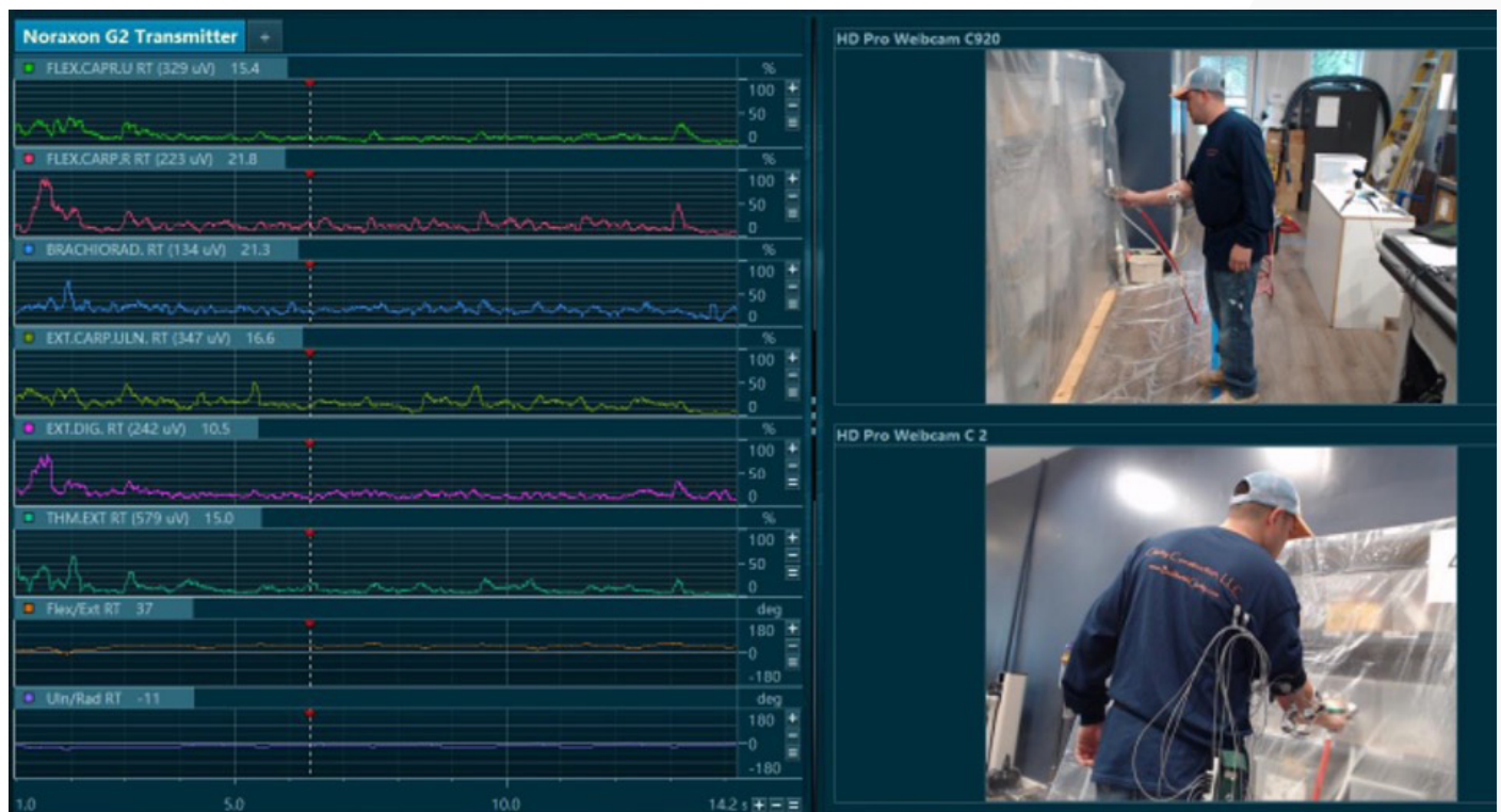
Sample EMG measurement also shows simulated painting.
