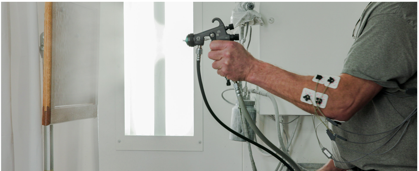
A painter's muscle effort is being measured as he uses the Stellair air spray gun during dynamic arm movement testing.
