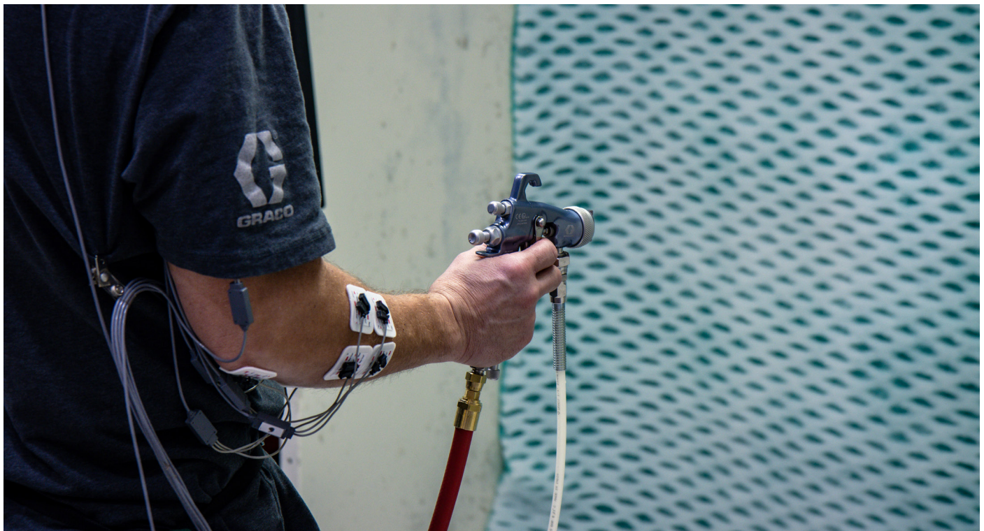
EMG measurements are made as a painter participates in the test.
