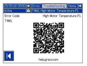
There are three types of errors that can occur. Errors are indicated on the display as well as by the light tower (optional).
