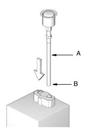
2. Install suction tube assembly to gear pump and motor assembly. Hand tighten securely.
