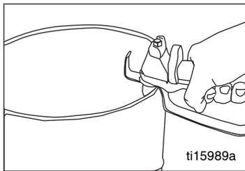
4. Re-engage gun trigger lock and turn Prime/Pressure Relief Valve (PR Valve) to the open (priming) position to relieve residual pressure.
