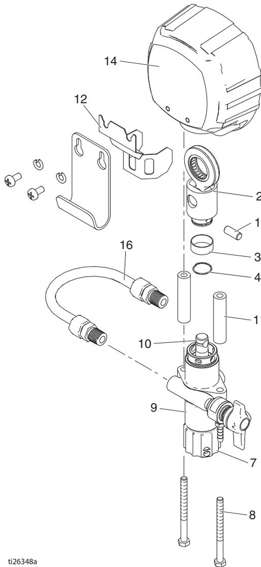
1. Un-thread and remove suction nut from the fluid pump body (8).
