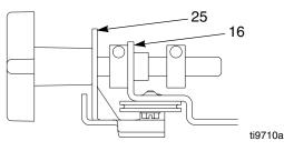
Tighten front spacer (56) until flush to front of tensioning bracket (16). Tighten back spacer (56) 3/8 in. from tensioning bracket.
