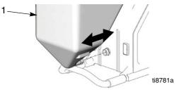
6. Use 3/8 in. socket to remove screw (36) from hose bracket (27).
