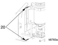
10. Slide motor tray (32) out of slots in base (2) to remove motor and tray from sprayer.
