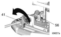
5. Loosen hopper fitting by hand to remove hopper (1).
