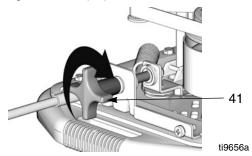
8. To set pressure, tighten knob (41) until back of bracket (25) is approximately 1/2 in. from front of tensioning bracket.
