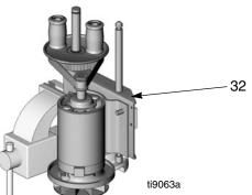
Use 9/16 in. wrench to loosen two mounting screws
