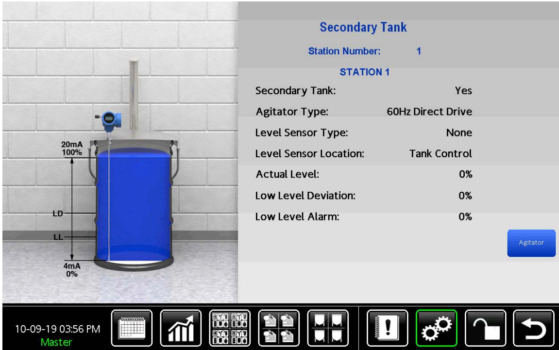
Figure 72 Secondary Tank Screen
