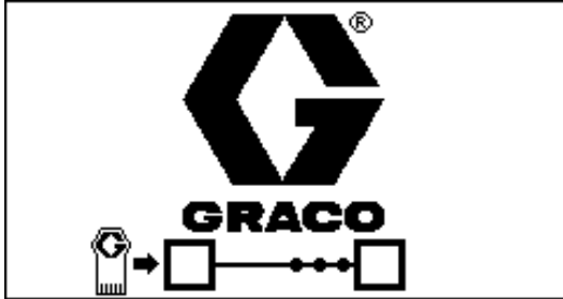
Communications with other modules established.
