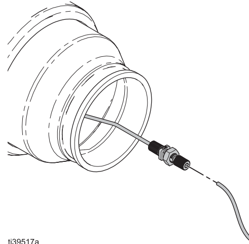
FIG. 12. Non-Electrostatic Fiber Optic Bulkhead Connection
