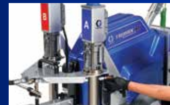
1) Remove retaining clamps and pressure transducer connections
