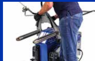
3) Remove ProConnect Pumping System
